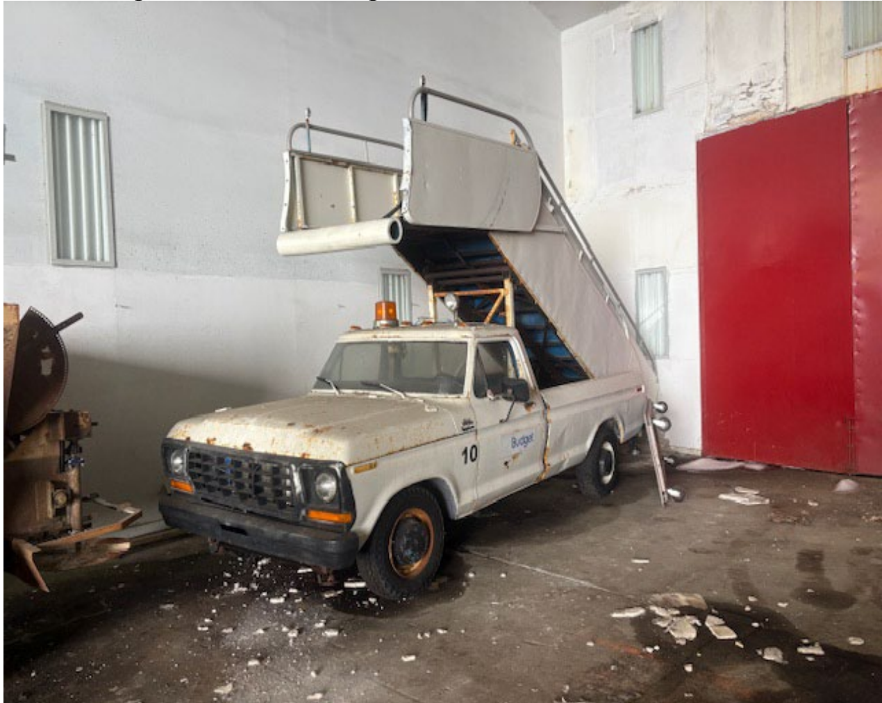
Ford F150 portable stairs not operational
